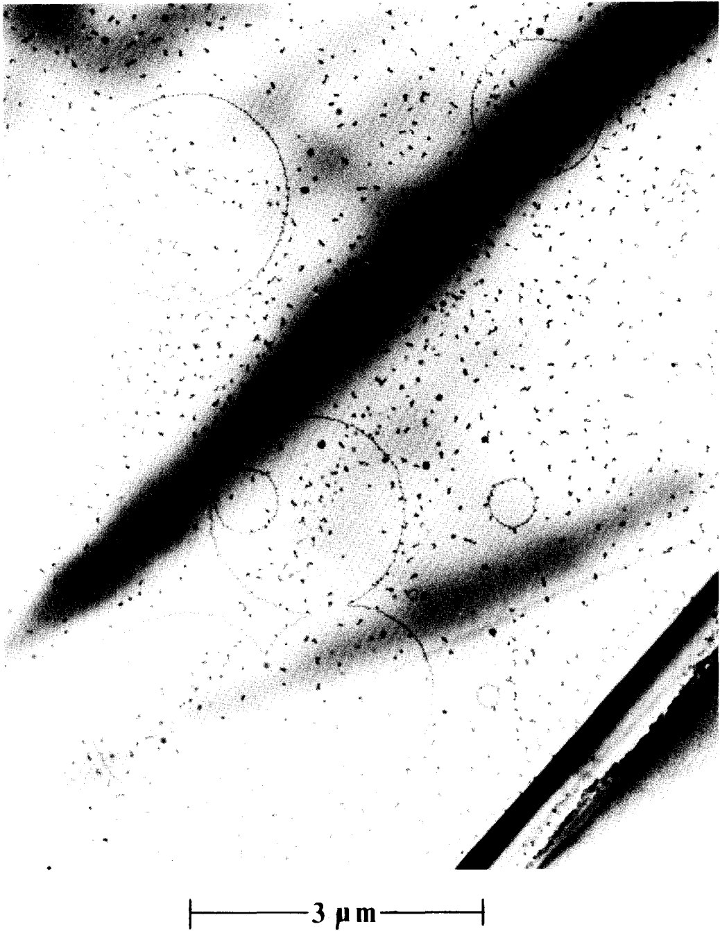
FIG. 5. Etch loops produced by oxidation at 680°C in 0.2 atm O 2 for 10 min, with WO 3 catalyst particles initially deposited on surface.
